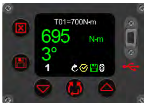
FIGURE 52 – Audit Torque target result (showing achieved torque and output (bolt) movement in degrees)
