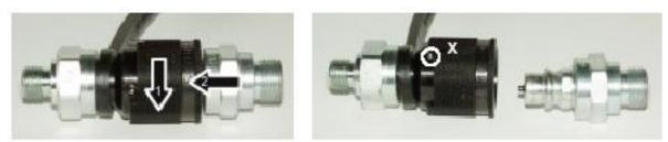
In position X, retract sleeve – plug and socket are uncoupled - the device is coupled in reverse order. The devices can only be coupled if the hose lines are **depressurized**. The supplied dust caps are used to protect the couplers against dirt.
