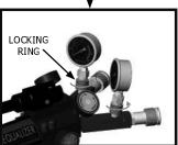
wish to pressurise have been bled and are free from air and leaks. Connect the pump into the systems using the screw connectors supplied with the pump, push the male and female connectors together fully and rotate the locking rings clockwise until fully tight.
